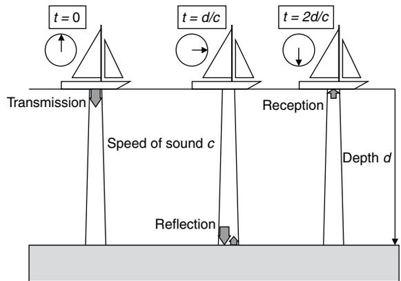
**Fig. 1.2** Measurement of water depth using the pulse–echo principle. The depth is worked out by measuring the time from transmission of the pulse to reception of the echo. The speed of sound must be known.
