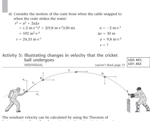
Pythagoras, i.e.  $v_{res}^2 = v_y^2 + v_x^2$  at each point. Note that the horizontal component of the velocity ( $v_x = u_x$ ) remains constant throughout the motion of the ball.
