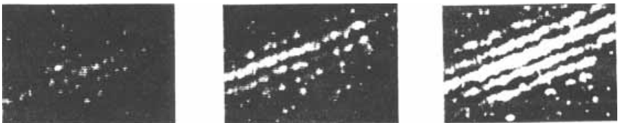
Fig. 1.3 Gradual genesis of an electron interference pattern in a double-slit experiment, with electrons reaching the detector one at a time. (Adapted with permission from ref. 5.)
