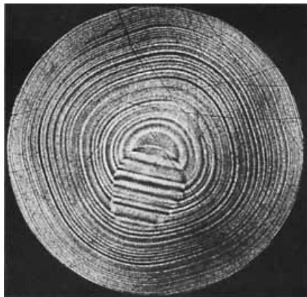
Figure 1.6. Transverse section of a \text{Ba}_2\text{NaNb}_5\text{O}_{15} crystal whose rotational striations form concentric closed loops. The striations are caused by temperature fluctuations in the melt. From Hurlé (1993).
