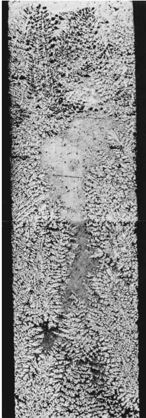
Figure 1.1. Longitudinal section of the quenched interface of the Zn-27%Al alloy. From Ayik et al. (1986).
