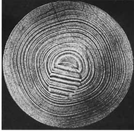
Figure 1.6. Transverse section of a \text{Ba}_2\text{NaNb}_5\text{O}_{15} crystal whose rotational striations form concentric closed loops. The striations are caused by temperature fluctuations in the melt. From Hurle (1993).
