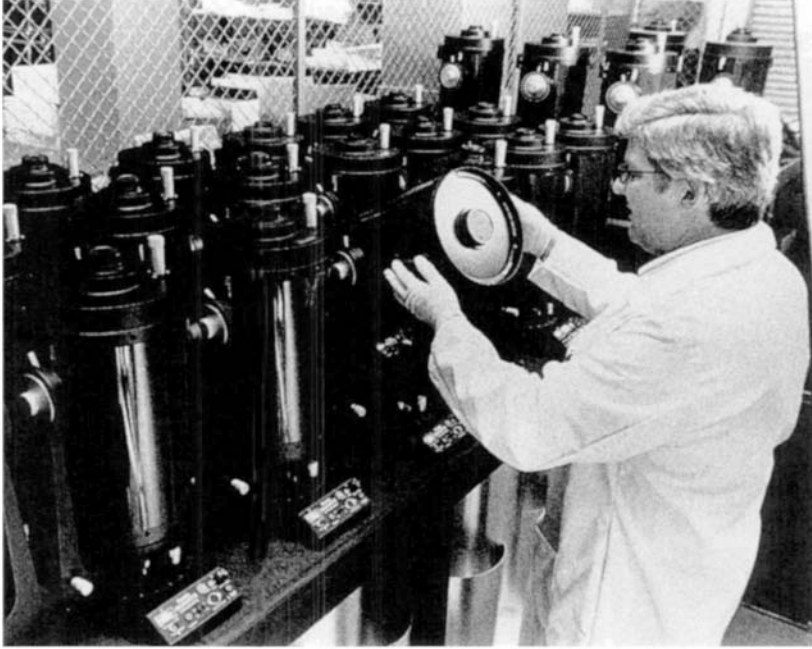
Figure 1.5. Production of 20-cm S-C Telescopes. Each of the 350–500 parts of the instrument is inspected and tested prior to assembly and then the overall system is checked before shipping. Photo courtesy of the Meade Instruments Corporation.
