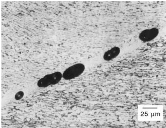
Figure 1.18. Voids formed within a shear band in Ti-6Al-4V. (Reproduced from Grebe et al. 1985. Copyright 1985 by the Minerals, Metals and Materials Society and ASM International.)
