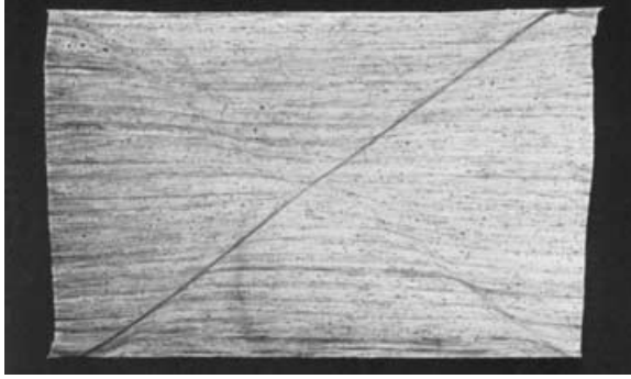
Figure 1.15. Adiabatic shear band formed in a compression specimen of 7039 Al at a strain rate of 8 \times 10^3 \text{ s}^{-1} . Total strain is 0.26. (Reproduced from Wulf 1978, with permission from Elsevier Science.)
