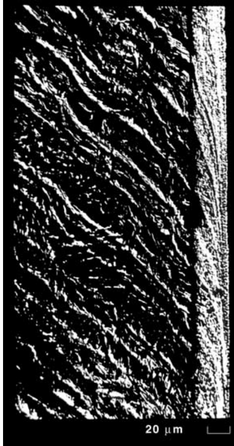
Figure 1.3. Adiabatic shear band in a Ni-Cr steel alloy. Band formed from a punch driven explosively through the specimen. White lines are bands of chemical inhomogeneity and were horizontal before punching. (Reproduced from Moss 1981, with permission from Kluwer Academic/Plenum Publishers.)
