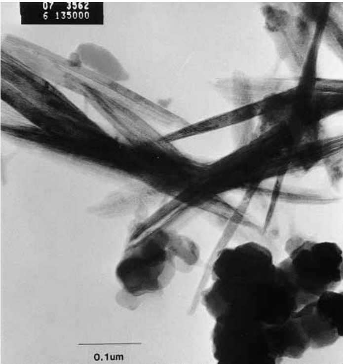
Plate 1.19. Transmission electron micrograph of synthetic goethite laths formed from controlled oxidation of an initially anoxic Fe^{2+}/Fe^{3+} suspension (Taylor et al. , 1987). (Photo: B. Maher).
