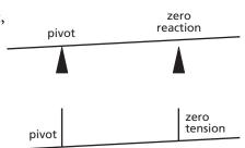
When a suspended rod is about to tilt about one support, the tension at the other support is zero.
