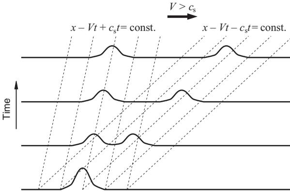
**Figure 1.1** Time evolution of wave equation from d'Alembert's solution for the case of a background flow  $V > c_s$ , showing the two families of characteristics (dashed).
