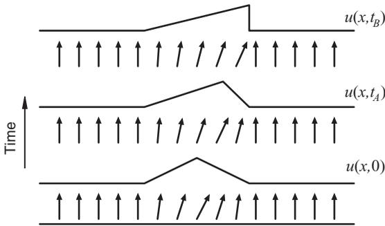
**Figure 1.2** Development of a discontinuous solution of Burgers' equation. Arrows indicate the slopes of the characteristics.
