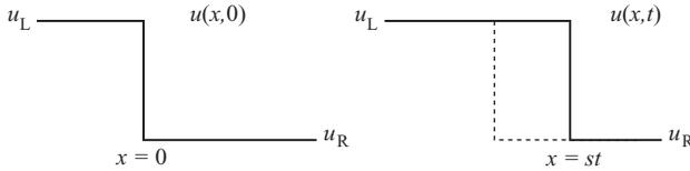
**Figure 1.4** Discontinuous solution to Burgers' equation for a change of state  $u_L \rightarrow u_R$  propagating at a speed  $s$ , for  $t = 0$  (left) and  $t > 0$  (right).
