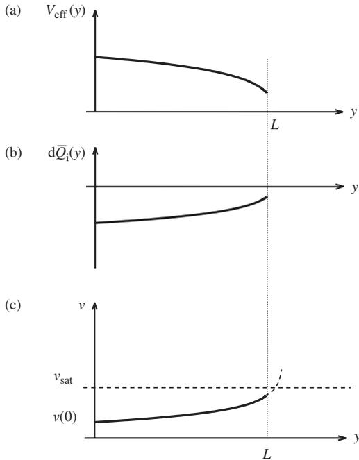
**Figure 1.5** The variation of (a) the effective channel voltage, (b) the corresponding inversion charge and (c) the velocity of electrons along the channel for a transistor operating in the resistive (no pinch-off) region.
