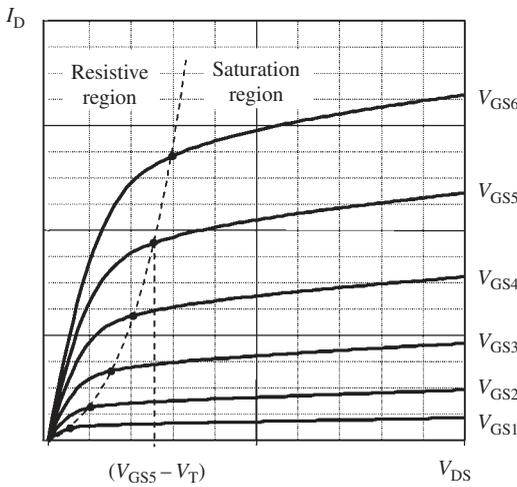
**Figure 1.8** The output characteristic curves of a typical NMOS transistor. The border between the resistive region and the saturation region corresponding to  $V_{DS} = (V_{GS} - V_T)$  is plotted as a dashed line.
