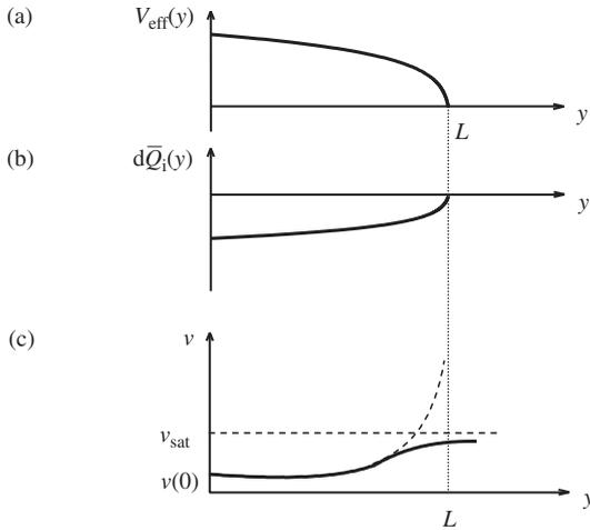
**Figure 1.4** The variation of (a) the effective channel voltage, (b) the corresponding inversion charge and (c) the velocity of electrons along the channel for a transistor pinched-off at the drain end of the channel.
