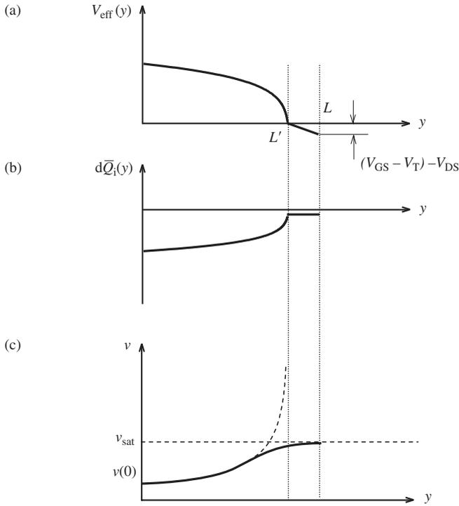
**Figure 1.6** The variation of (a) the effective channel voltage, (b) the corresponding inversion charge and (c) the velocity of electrons along the channel for a transistor pinched-off before the drain end of the channel.
