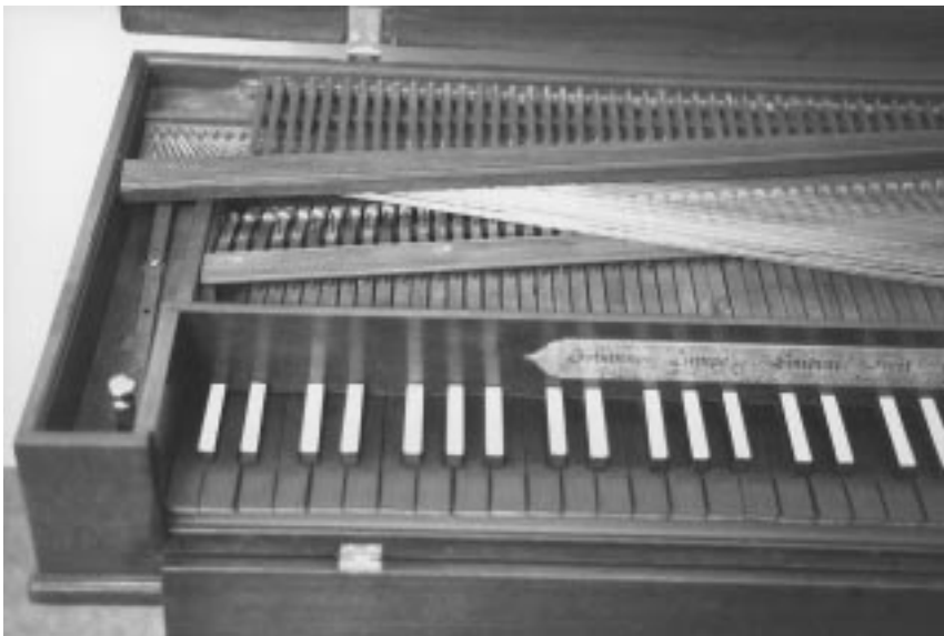
Figure 1.4b Detail of Zumpe piano showing (inside the case, to the left) the sustaining handstop which raises the bass dampers from the strings, the small, leather-covered hammers and (at the top of the photograph) the wooden levers on which the dampers are mounted.
