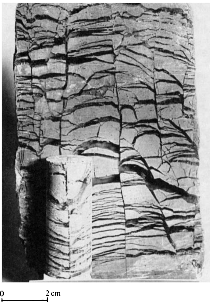
Figure 1.1 Frozen clay showing typical ice layers (or 'lenses'). This ice is mainly from water which is drawn to the freezing zone, and is the cause of the expansion constituting frost heave. See also Chapter 8, Figure 8.12. The ice layers vary greatly in size and form, from soil to soil. Photograph from Williams (1986).
