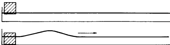
Fig. 1.3 Diagram of Scott Russell's experiment to generate a solitary wave.
