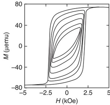
**Fig. 1.1** Hysteresis curve of the magnetization as a function of the applied field for a CoPtCrB thin film. Multilayer Co/Pt is used in memory storage. Reprinted from Carpenter *et al.*, *Phys. Rev. B* **72**, 052410 (2005).
