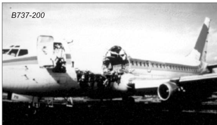
Figure 1.1. In-flight separation of an upper section of the fuselage of a B737-200 aircraft in 1988 attributed to corrosion and fatigue.
