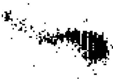
Figure 1.1 The two-dimensional projection of a track produced when a 54 keV X-ray was absorbed in a mixture of argon (90%), CH 4 (5%), and trimethylamine (5%) at 2 atm. This particular track is \simeq 14 mm in length.
