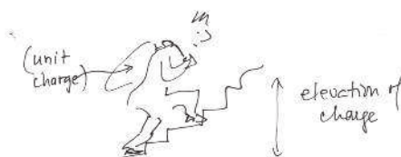
Figure 1N.3 Voltage is work to raise a unit charge from one level to a higher level (or “potential”).
