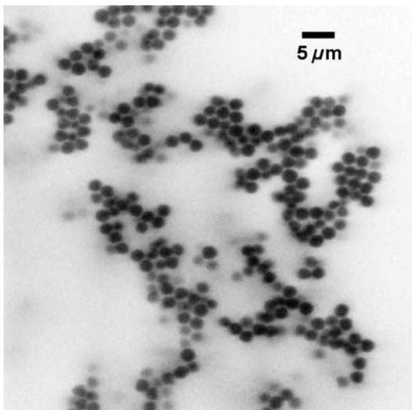
Figure 1.4 Image of a colloidal gel, taken with confocal microscopy. The particles are  $2\ \mu\text{m}$  diameter and aggregate due to the depletion force which is caused by adding small polymers to the solvent [14]. Image from Gary Hunter and Eric R. Weeks. See Chapter 3 for more information about colloidal gels.
