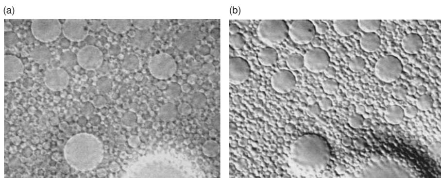
Figure 1.1 (a) Image of an oil-in-water emulsion taken using brightfield microscopy. The picture is  $\sim 60 \mu\text{m}$  wide. (b) Image of the same field of view taken using differential interference contrast microscopy. This form of microscopy produces a fictitious three-dimensional appearance; in reality, these are the cross-sections of spherical droplets. *Note:* the contrast in both pictures has been enhanced for better appearance.
