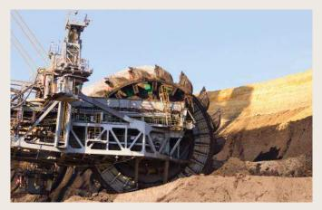
Figure 1.0 A giant bucket wheel excavator in use in an open-pit mine.
