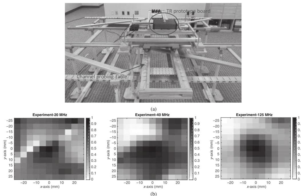
**Figure 1.7** Spatial focusing effect of TR wideband system prototype: (a) TR wideband system prototype and (b) experiment results.
