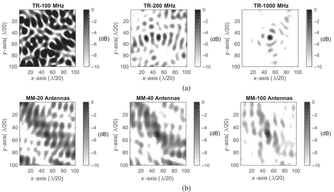
Figure 1.6 Spatial focusing effect of both systems: (a) TR wideband system and (b) massive MIMO system.
