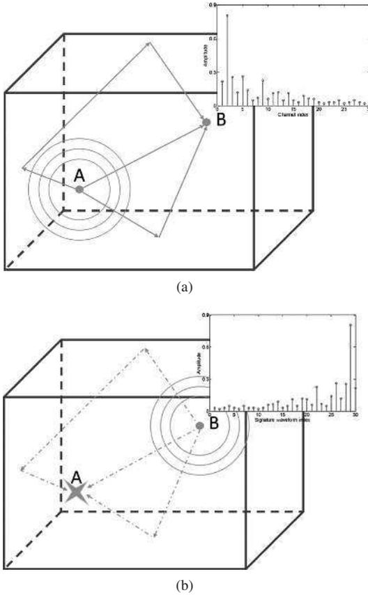
**Figure 1.4** An illustration of time reversal: (a) channel probing phase and (b) data transmission and focusing phase.
