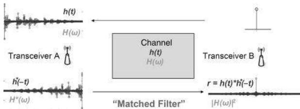
**Figure 1.3** The time-reversal signal processing principle.
