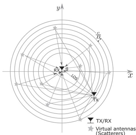
**Figure 1.1** Illustration of multipath as virtual antenna.
