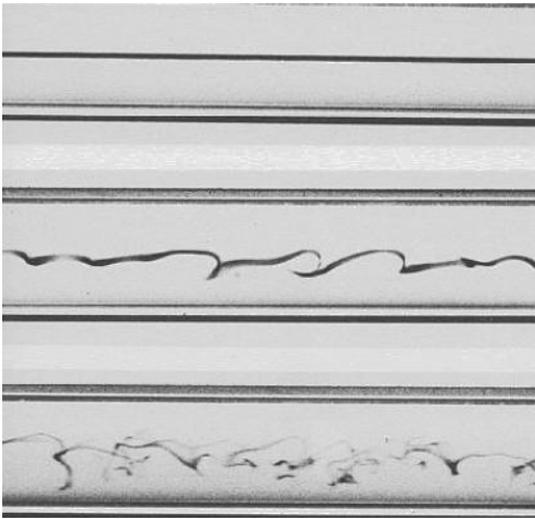
Figure 1.5 Repetition of Reynolds' dye pipe experiment (van Dyke, 1982).
