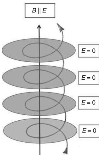
Figure 1.4 Trajectory of electron motion in electromagnetic field.
