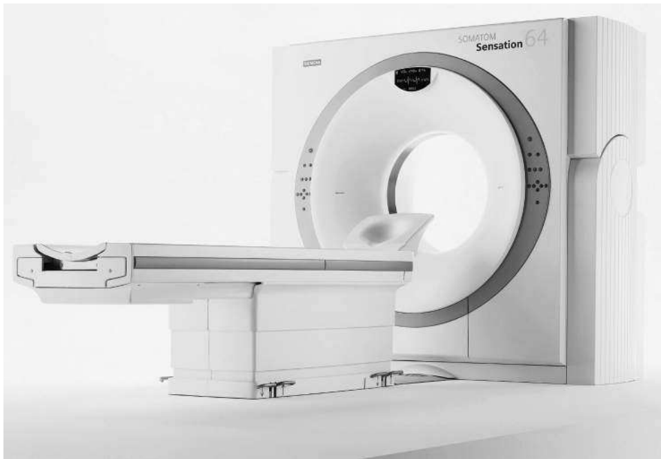
Figure 1.1 A typical CT scanner consisting of a gantry housing the rotating x-ray source and detector arrays. The patient table is moved into the aperture in the gantry for imaging.
