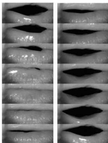
Figure 2 A cycle of motion of a brass player's lips (frontal view, obtained with a high-speed camera and transparent mouthpiece).
