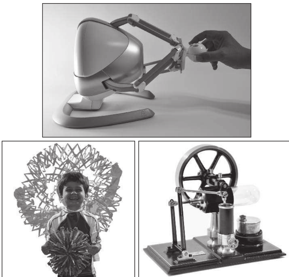
Figure 1.4 Some devices that operate under holonomic constraints. (Top) The Falcon haptic game controller by Novint Technologies Inc. (Bottom Left) The Hoberman Sphere © 1993 Charles Hoberman. (Bottom Right) A Stirling engine by Wiggers Stirling HeiBluft Modellbau. All images © 2016 Vincent De Sapio.
