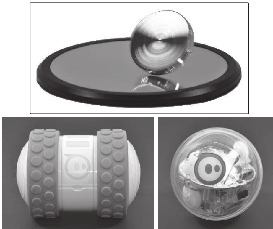
Figure 1.5 Some devices that operate under nonholonomic constraints. (Top) Euler's Disk by Toymsmith. (Bottom Left) Ollie by Sphero Inc. (Bottom Right) Sphero SPRK edition by Sphero Inc. All images © 2016 Vincent De Sapio.
