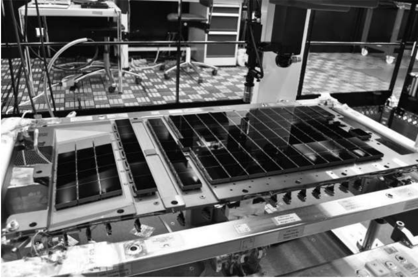
Figure 4. Gaia focal plane assembly. Groups from left to right: 12 RVS CCDs, 7 RP CCDs, 7 BP CCDs, 62 astrometric CCDs and 14 sky mapper CCDs. The two most extreme CCDs in the corner are for the Basic Angle Monitor and the one out of the row of astrometric CCDs together with the one most to the right in the middle of the focal plane are for wavefront sensors (the wavefront sensor is missing still in this picture). Copyright Airbus DS
