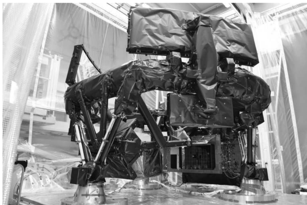
Figure 2. Gaia payload module at the time of vibration testing. Copyright Airbus DS
