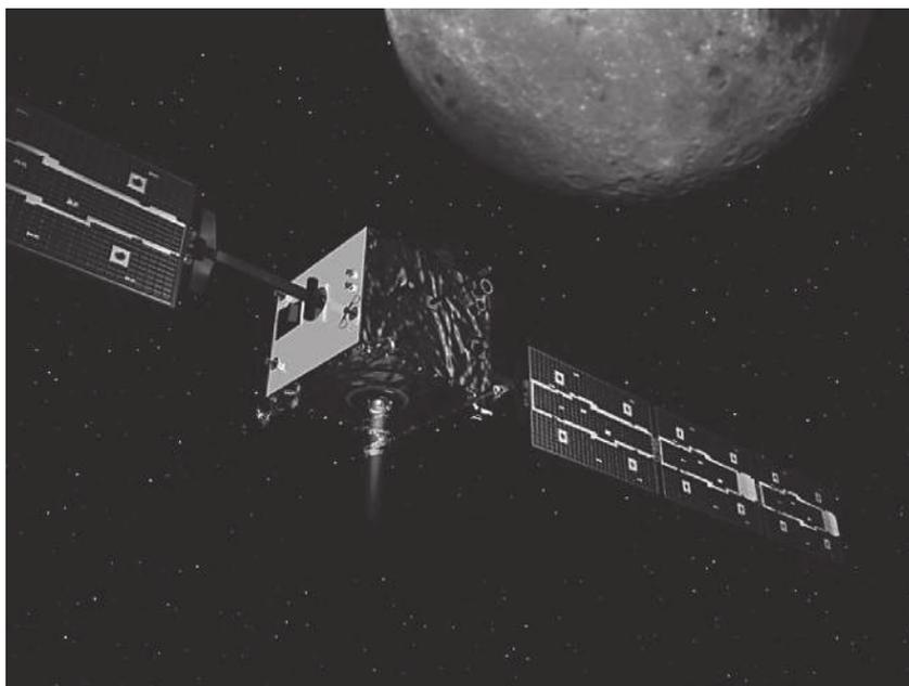
**Figure 1.3** SMART-1 (Small Missions for Advanced Research in Technology) was an ESA mission (launched in 2003 and deliberately crashed into the Moon's surface in 2006) which orbited around the Moon. It was propelled by a Hall-effect thruster (visible on this image at the bottom of the satellite). Image: ESA/SMART-1.
