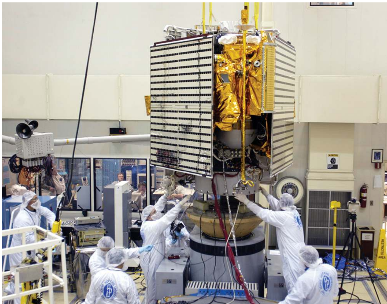
Figure 1.3. View of the MESSENGER spacecraft during vibration testing at the Johns Hopkins University Applied Physics Laboratory. The solar arrays (mirrored surfaces) are stowed in their positions at the time of launch. Also visible are the Magnetometer boom (center), similarly in its stowed position, and thermal blankets (gold).
