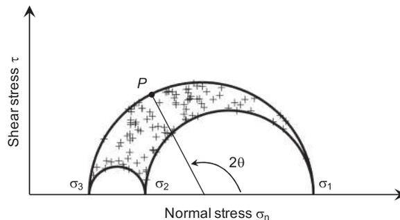
**Fig. 1.2** 3-D Mohr diagram, showing principal stresses,  $\sigma_1 \geq \sigma_2 \geq \sigma_3$ . Symbols represent the state of stress on 100 randomly oriented fractures. Point  $P$  defines the state of stress for a plane whose normal is co-planar with the maximum and minimum principal stress axes and that makes an angle  $\theta$  with respect to the maximum principal stress axis.
