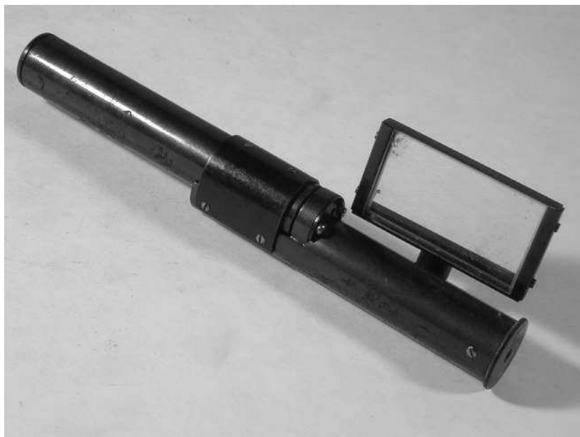
1.2 A heliostat designed by Francis Galton. © UCL Galton Collection.
