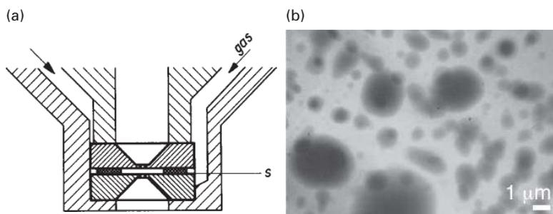
**Figure 1.2.** Environmental chamber closed with thin windows. (a) Two aperture holders support thin films and are placed face to face in the upper pole shoe of the objective lens. A thin film between the aperture holders (s) serves as a spacer of about  $5\ \mu\text{m}$  thickness. (b) Electron micrograph of water droplets condensed on the support film at a pressure of 0.13 bar. From Ref. 12 with kind permission from Springer Science+Business Media.
