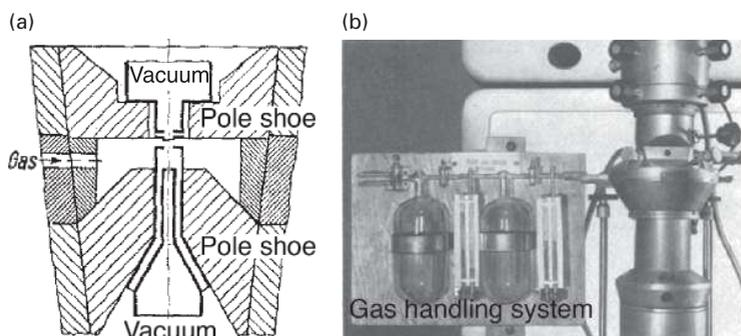
**Figure 1.1.** Transmission electron microscope with differentially pumped environmental chamber for imaging specimens at higher pressures. (a) The specimen in a gaseous environment is separated from the high vacuum of the electron column via pump-limiting apertures. The apertures are placed on the pole pieces (shoes) of the objective lens. (b) Photograph of electron microscope with gas handling system. From Ref. 5 with kind permission from Springer Science+Business Media.
