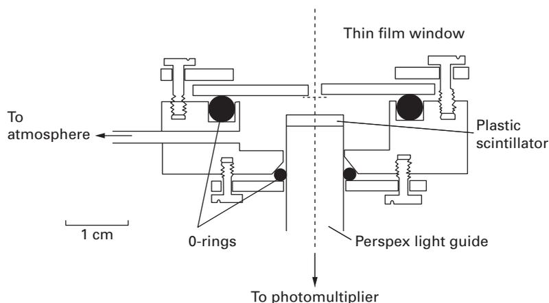
**Figure 1.5.** Environmental cell for a scanning electron microscope. From Ref. 41, © IOP Publishing. Reproduced with permission. All rights reserved.
