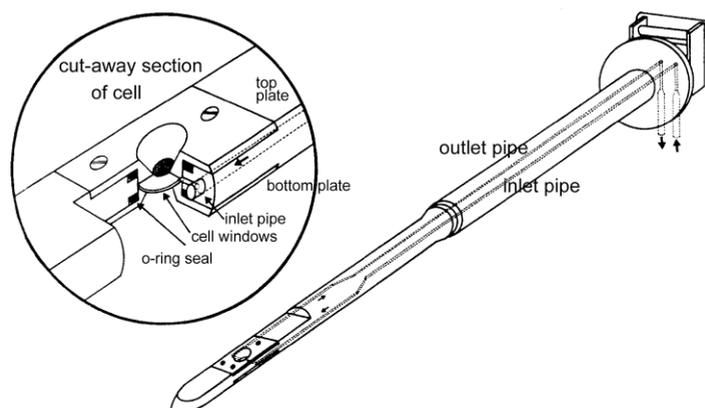
**Figure 1.3.** Early design of an environmental cell integrated in a side entry sample holder, with access pipes for gas flow from outside the electron microscope. Reprinted from Ref. 14, Copyright 1973, with permission from Elsevier.
