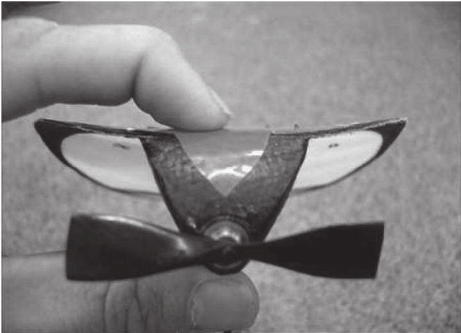
Figure 1.1 A 10cm-span fixed-wing MAV (Courtesy of Michall Sytsma)
