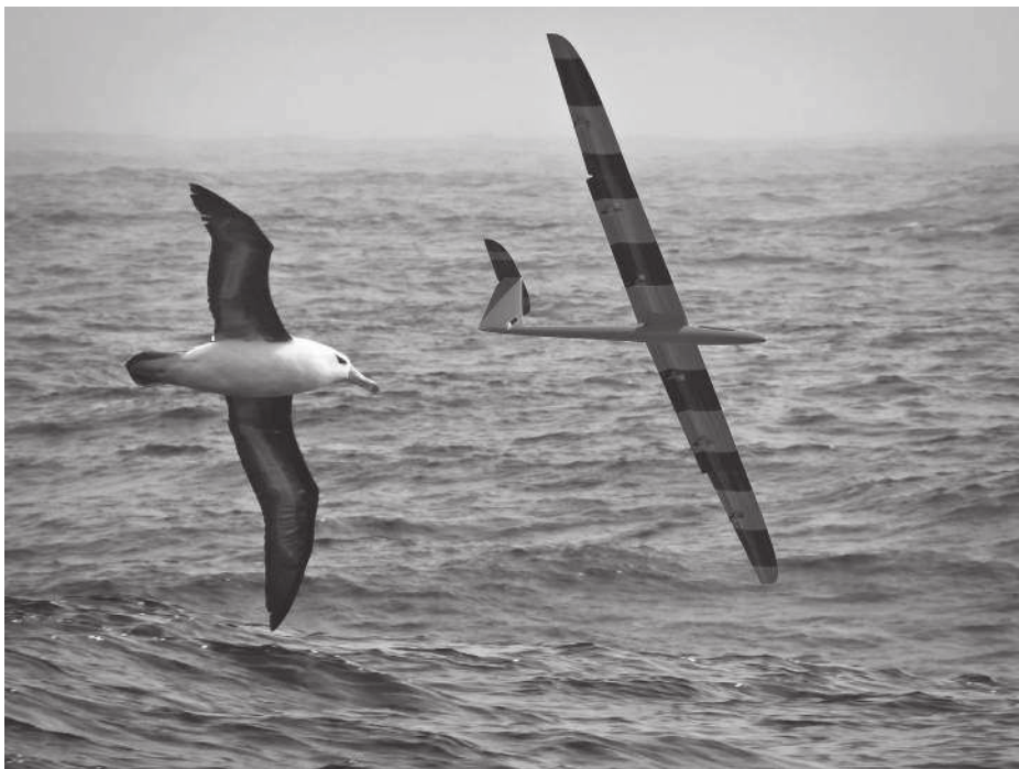
Figure 1.5 Long-endurance mini-UAV concept inspired from the albatross flight (Courtesy Philip Richardson, 2012)
