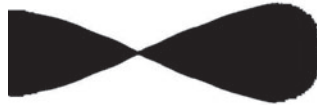
Figure 1.4 A hypothetical breakup mode without satellite formation: an engineering dream that is unfulfillable.
