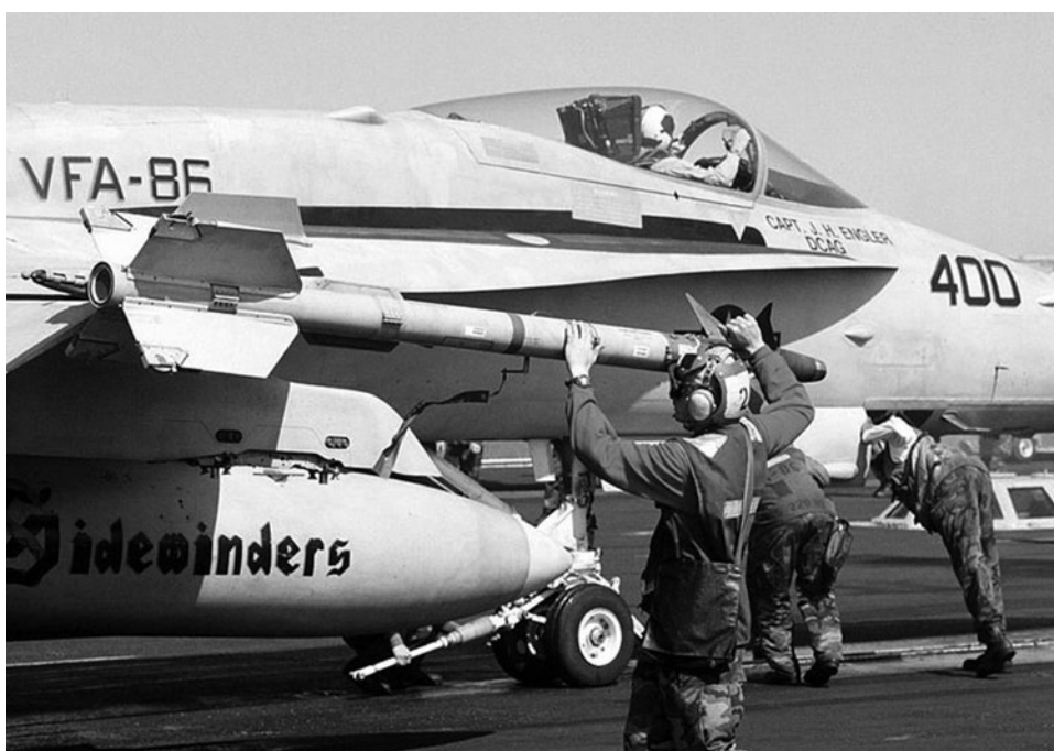
Figure 1.7. U.S. Marine Corps Lance Cpl. Leander Pickens arms an AIM-9 Sidewinder missile on a FA-18C Hornet. Image courtesy of U.S. Navy ID 980220-N-0507F-003.
