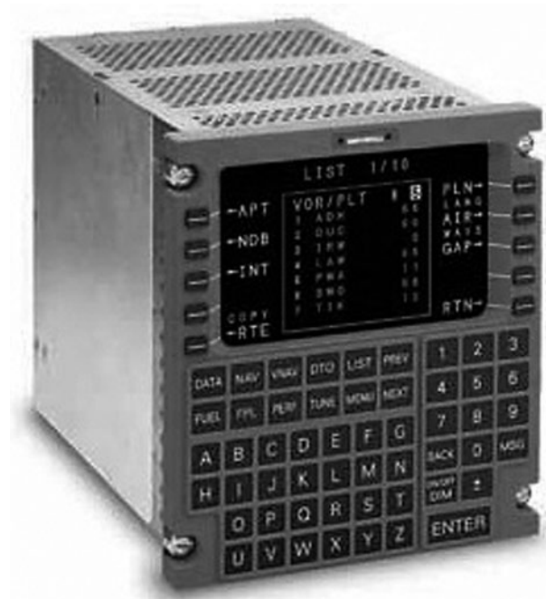
Figure 1.5. A control display unit (CDU) used to control the first flight management system (FMS), UNS-1. Image courtesy of FAA Instrument Flying Handbook, FAA-H-8083-15B.
