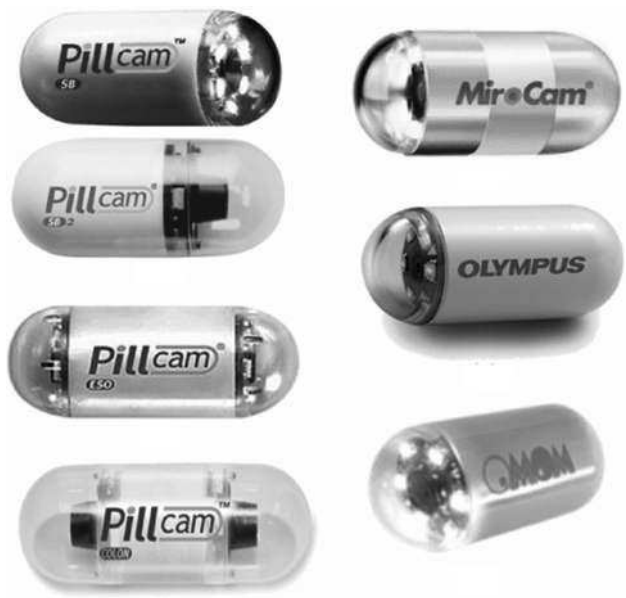
Figure 1.1 Examples of commercially available camera capsules for GI tract visualization [26].
