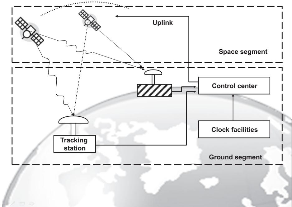
Figure 1.1 GNSS space and ground segments.
