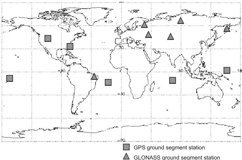
**Figure 1.6** Ground segment networks for GPS (after [1]) and GLONASS (after [3]).
