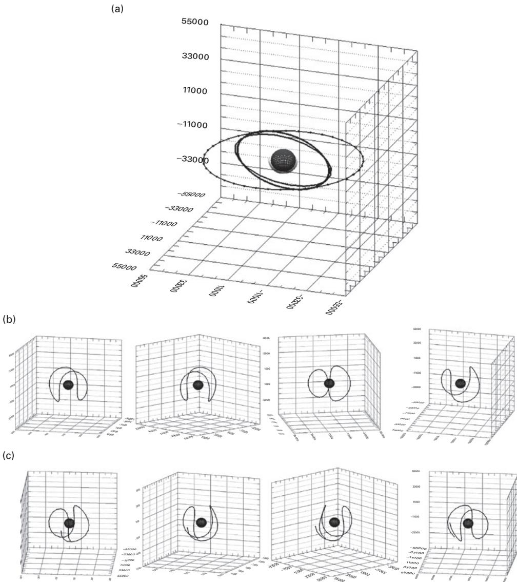
**Figure 1.4** (a) GPS, GLONASS, and GEO orbits in ECI; (b) GPS orbit in ECEF; (c) GLONASS orbit in ECEF.
