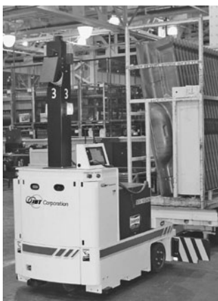
Figure 1.2 Tug AGV (JBT Corporation, Philadelphia, USA). These laser guided vehicles are used in factories to move materials from place to place.
