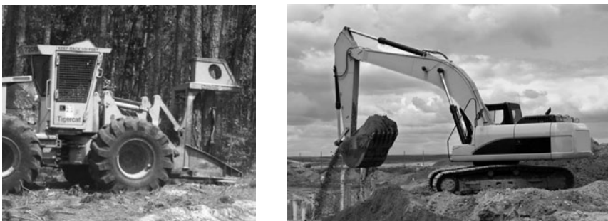
Figure 1.7 Field Robots. Field robots must engage the world exactly as it exists. (Left) Semi-automated fellerbunchers similar to this one have been designed to gather trees. (Right) Automated excavators have been prototyped for mass excavation applications—where large amounts of dirt are loaded over short time periods.
