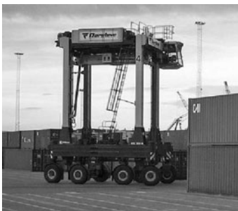
Figure 1.3 Straddle Carrier. Used to move containers to and from ships, automated versions of these vehicles are perhaps the largest AGVs in use today.
