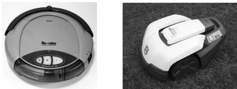
Figure 1.5 Floor and Lawn Care Service Robots. These kinds of mobile robots care about area coverage. They try to “visit” every place in some predefined area.
