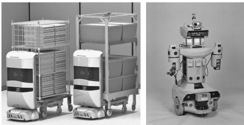
Figure 1.4 Health Care and Surveillance Service Robots. (Left) The Aethon Corp. “Tug” Vehicle is used to move food, linens, records, specimens, and biological waste in hospital settings. (Right) A surveillance robot like Robart might scan a warehouse for unwanted intruders on its regular rounds.
