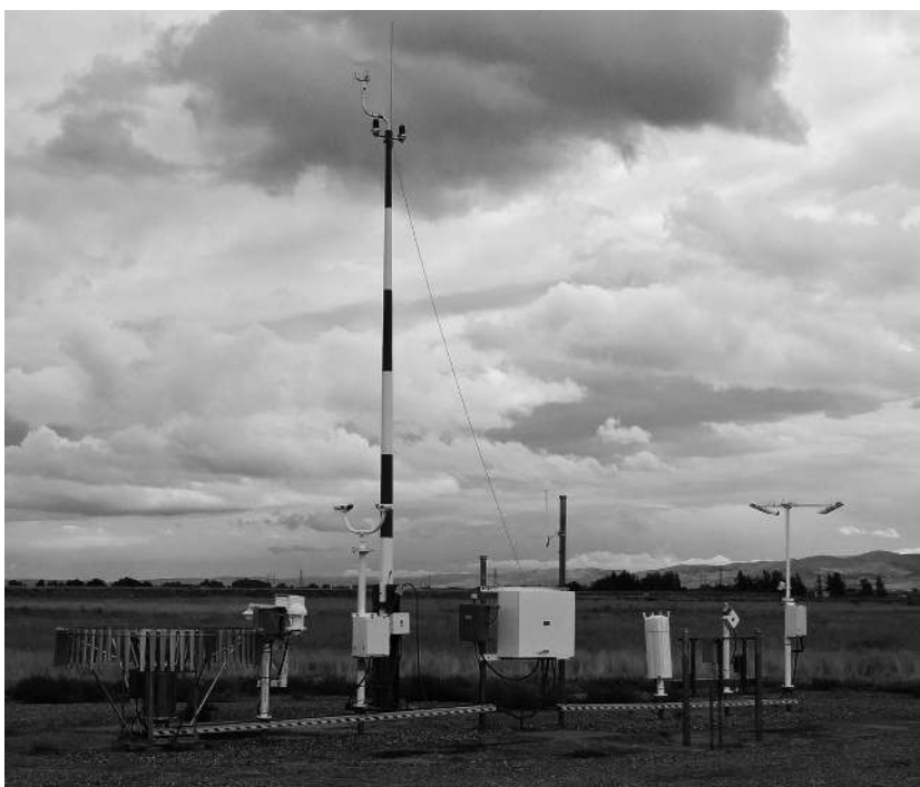
Figure 1.2. The U.S. National Weather Service Automated Surface Observing System (ASOS) sensor package located at Pocatello, Idaho ( 42^{\circ} 55' \text{ N} , 112^{\circ} 34' \text{ W} , 1356 m above MSL, WMO station no. 72578), October 2011. From left to right, the instruments shown are – heated tipping-bucket raingauge within wind shield: aspirated temperature and humidity sensors: present weather sensor: 10 m wind mast with heated ultrasonic wind sensor: data collection panel (big box): laser ceilometers: freezing precipitation sensor (little tilted box), and finally the visibility sensor. (Photograph by Gary Wicklund)
