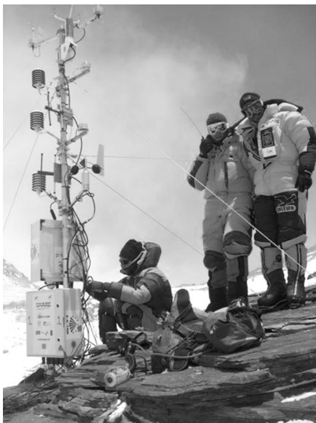
Figure 1.1. Installing the world's highest weather station at 8000 m above sea level on the south col of Mt Everest, May 2011. The summit is 8850 m. Observations are updated hourly on the web – http://share-everest.it/SHAREEverest2011MeteoData/SouthCol/sensorSouthCol.html (Photograph courtesy of the Ev-K2-CNR Committee archive)
