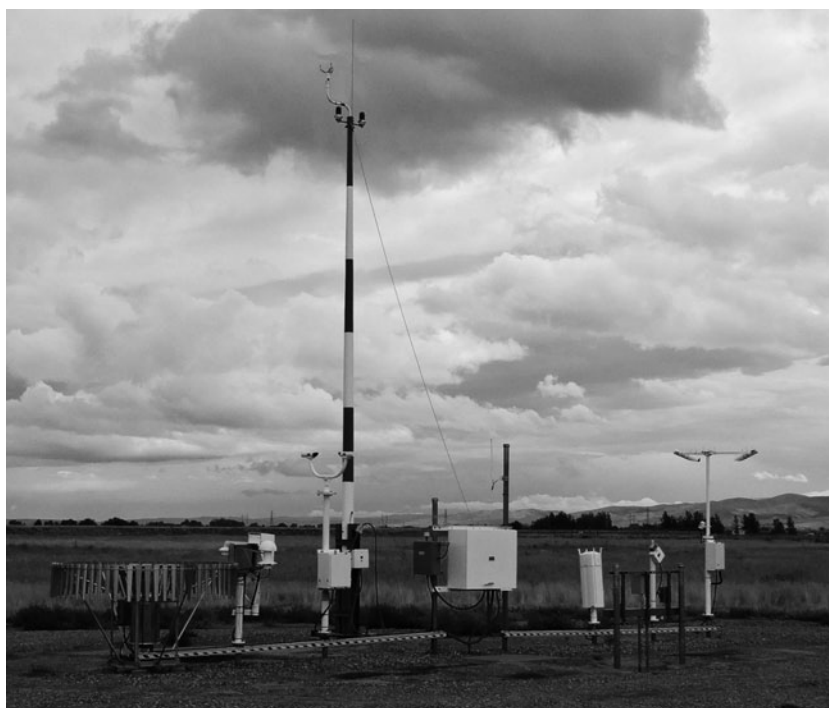
Figure 1.2. The U.S. National Weather Service Automated Surface Observing System (ASOS) sensor package located at Pocatello, Idaho ( 42^{\circ} 55' N , 112^{\circ} 34' W , 1356 m above MSL, WMO station no. 72578), October 2011. From left to right, the instruments shown are – heated tipping-bucket raingauge within wind shield: aspirated temperature and humidity sensors: present weather sensor: 10 m wind mast with heated ultrasonic wind sensor: data collection panel (big box): laser ceilometers: freezing precipitation sensor (little tilted box), and finally the visibility sensor. (Photograph by Gary Wicklund)
