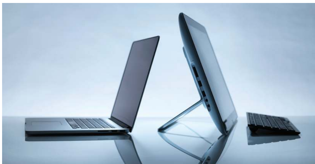
A laptop (left) and an all-in-one desktop computer with all components mounted inside the back of the screen (right)
