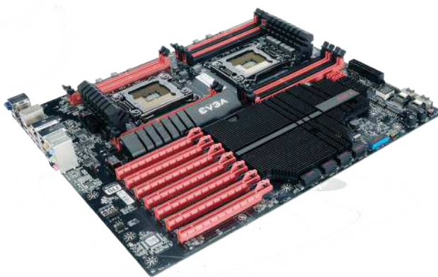
A multiprocessing motherboard with two processor sockets
