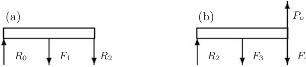
Figure 1.3. Free bodies of the simple model: (a) left bar, (b) right bar.
