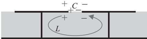
Fig. 1.5 Lumped LC model for EBG analysis.
