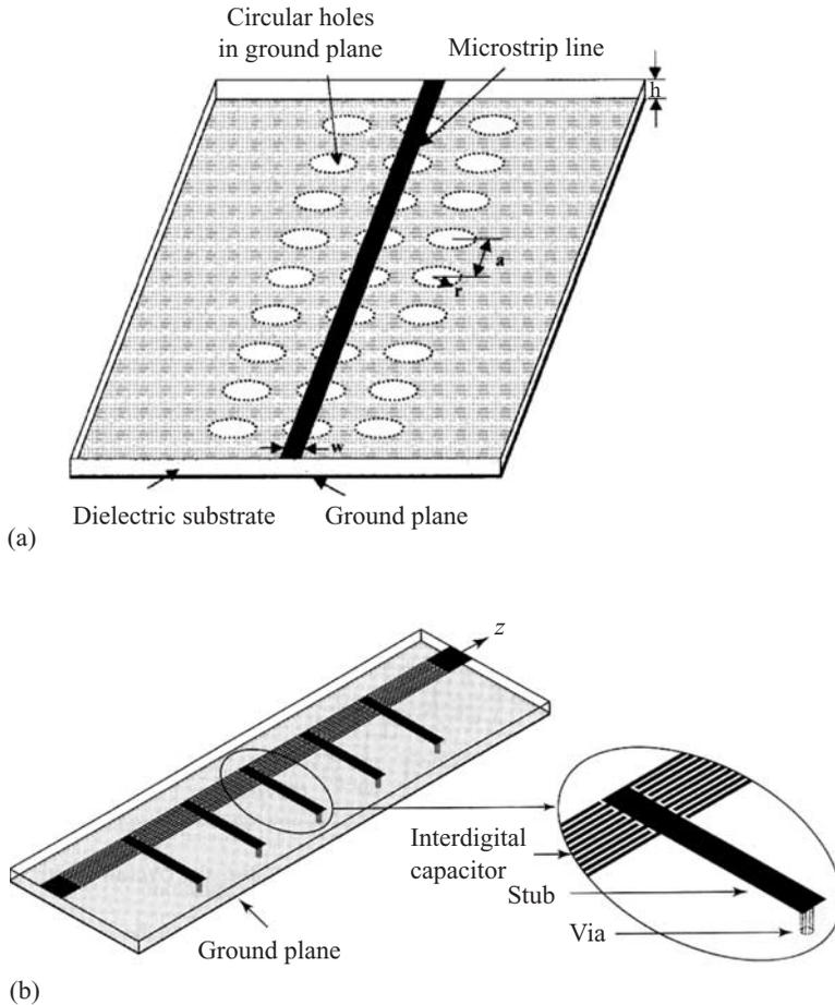
**Fig. 1.3** One-dimensional EBG transmission lines: (a) a microstrip line with periodic holes on the ground plane (from [9], © IEEE, 1998) and (b) a composite right- and left-handed transmission line (from [10], © Wiley-IEEE, 2005).
