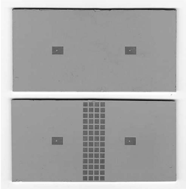
**Fig. 1.8** EBG substrate for surface wave suppressions: low mutual coupling microstrip array design (from [22], © IEEE, 2003).
