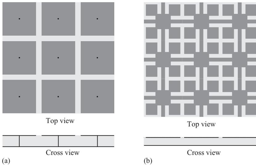
**Fig. 1.2** Two-dimensional EBG surfaces: (a) a mushroom-like surface and (b) a uni-planar surface.
