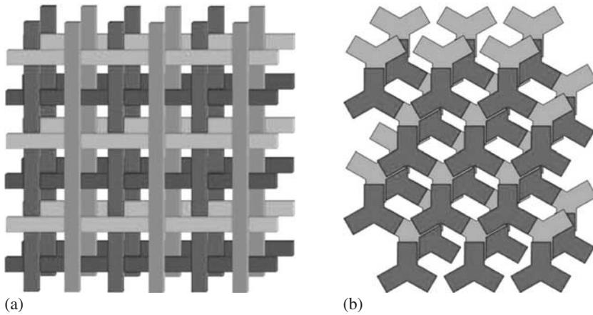
**Fig. 1.1** Three-dimensional EBG structures: (a) a woodpile dielectric structure and (b) a multi-layer metallic tripod array.
