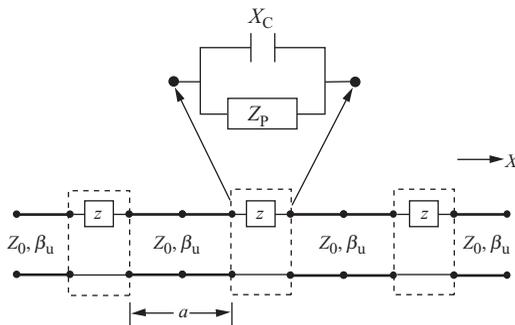
Fig. 1.6 Periodic transmission line method for EBG analysis (from [16], © Wiley InterScience, 2001).
