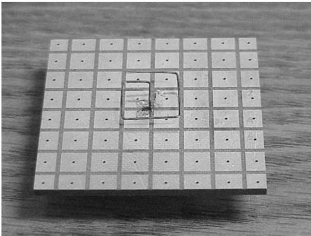
**Fig. 1.9** EBG substrate for a low profile curl antenna design (from [24] © Wiley InterScience, 2001).
