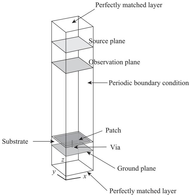
Fig. 1.7 Full wave FDTD model for EBG analysis.
