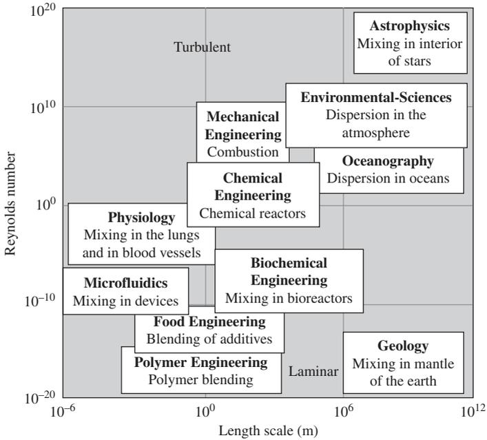
Figure 1.1 Spectrum of mixing problems. [Adapted from Ottino (1990).]
