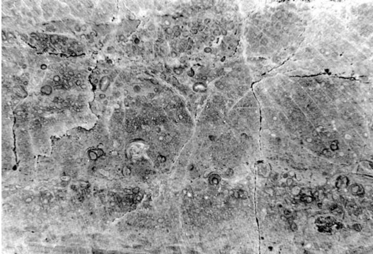
Figure 2.4. In this calcite block, previous fractures have been filled with dolomite, while more recent fractures remain partially open.
