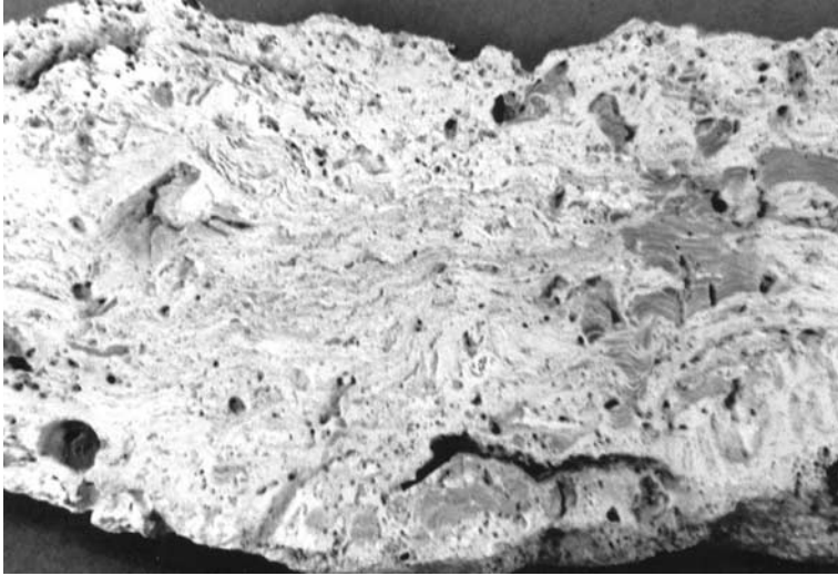
Figure 2.1. An extremely porous limestone from a Bermuda coral reef, approximately half-scale, containing shell fragments and many interstices with scales of up to a centimeter or so, courtesy of Professor L. Hardie.
