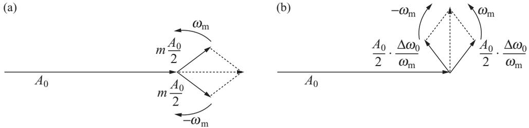
**Figure 1.2** (a) Amplitude-modulated carrier and (b) phase-modulated carrier
