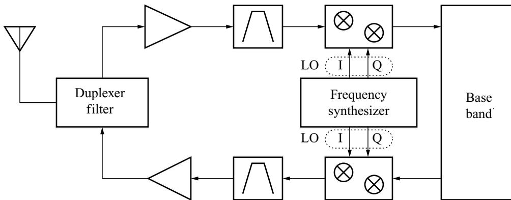
**Figure 1.1** Generic structure of a transceiver
