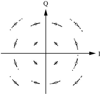
**Figure 1.7** A 16-QAM constellation affected by phase noise
