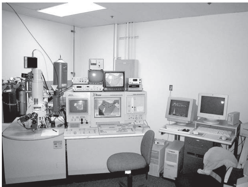
Scanning electron microscope equipped with a cathodoluminescence detector.
