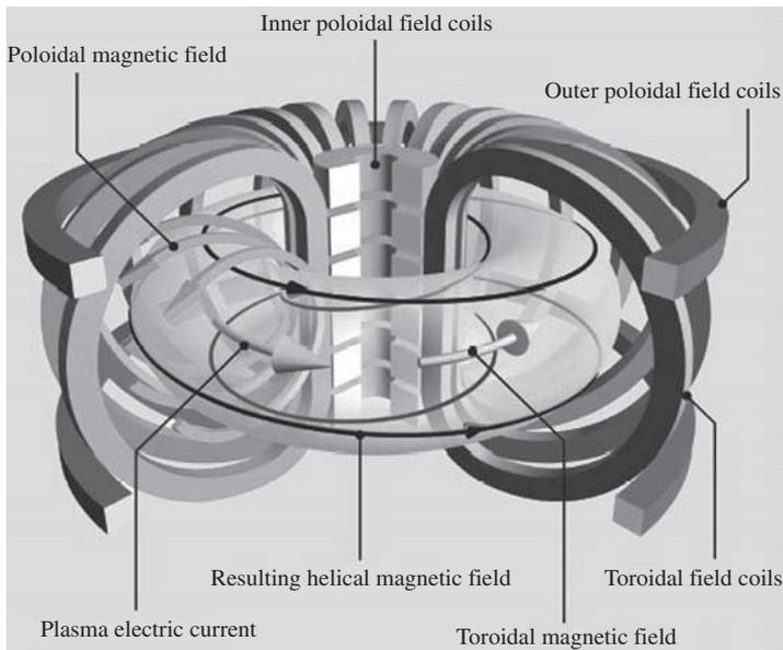
Fig. 1.1. Schematic representation of a *tokamak*. © EFDA-JET.
