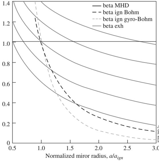
Fig. 1.2. Beta limits (ignition, stability and exhaust) vs. reactor size.
