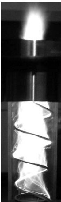
Figure 1–8. Gliding arc discharge stabilized in the reverse vortex (“tornado”) gas flow.
