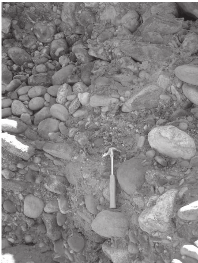
Figure 1.6 Fluvial gravels: the ingredients of a future conglomerate, Uranium Road, western Colorado. Hammer for scale. Some of the gravel pore spaces have been infilled by sand and mud, yielding a lower porosity and permeability but providing the cementing agents to convert the gravel to a conglomerate. The gravel is well rounded, as in a typical conglomerate, due to extensive abrasion in the stream that transported and then deposited it. Needless to say, this material is difficult to drill into and even more difficult to collect a sample of.
