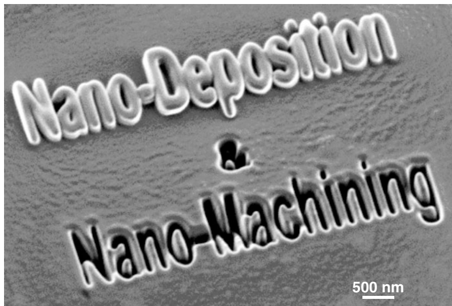
Figure 1.1 A typical SEM image showing the simultaneous milling and deposition capabilities of a two-beam FIB system. (Courtesy of Fibics Incorporated.)
